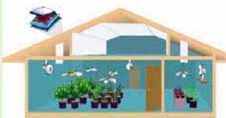
A single 1000-watt metal halide can grow enough mothers, clones, and vegetative plants to support 4000 watts of flowering HID light. This design allows pungent odors to waft upward before being evacuated via roof fans. A third area in the attic is used as a heat buffer in hot climates.
